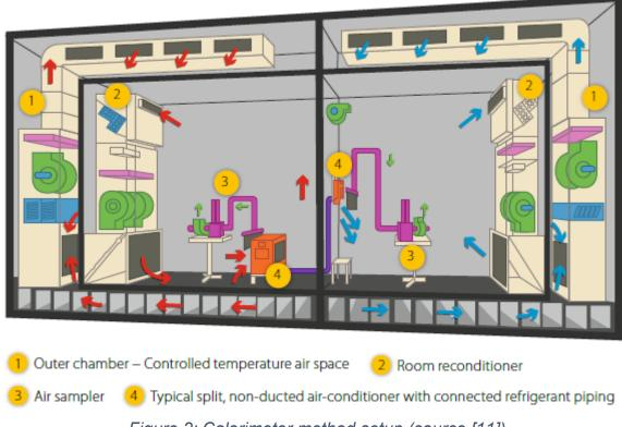
Figure 2: Calorimeter method setup (source [11])
